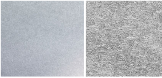
Left: Angel Hair Stainless Steel by Zahner. Above: "Vibration" finish by industry manufacturers. Right: The Zahner patented non-directional finishing system for manufacturing Angel Hair Stainless Steel.
